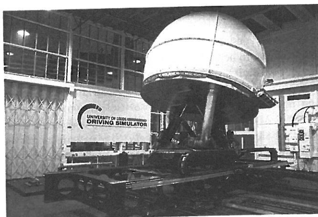
FIGURE 7.1 The motion system in the University of Leeds Driving Simulator.
